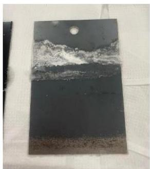
A single black panel is shown. The top portion of the panel is covered in a white, crystalline or powdery substance, indicating corrosion. |
